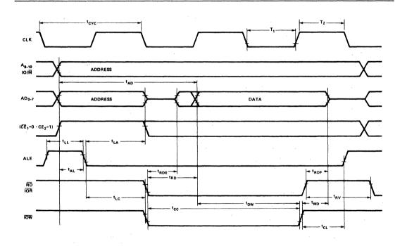
Figure 2. ROM Read and I/O Read and Write
